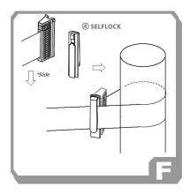
**③ SELFLOCK** should lock belt itself without **③ WALL SHOR** or in case of temporarily using.
